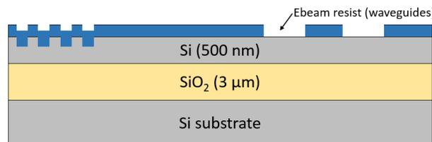
6. Deep Si ICP etch (500 nm etch depth)
