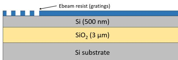
3. Shallow Si ICP etch (160 nm etch depth)
