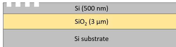
5. E-beam patterning for Silicon Etch 2 (GDS layers 3 & 4) – 500 nm etch
