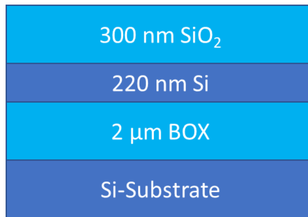
Figure 1 Sample layer stack of 300 nm \text{SiO}_2 on 220nm Si on 2 \mu\text{m} BOX on Si substrate
