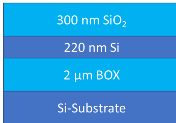
Figure 1 Sample layer stack of 300 nm SiO 2 on 220nm Si on 2 \mu m BOX on Si substrate
